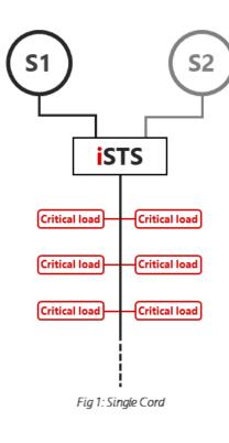
The configuration described by *Fig 1* is the typical application where there are two sources available for powering a critical item equipment/infrastructure and where it has only one power inlet receptacle. Reliability and redundancy can be improved by having a second source available to per the load in case one fails.
